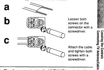
Plug the connector into the VHF/UHF terminal at the rear of the TV.
